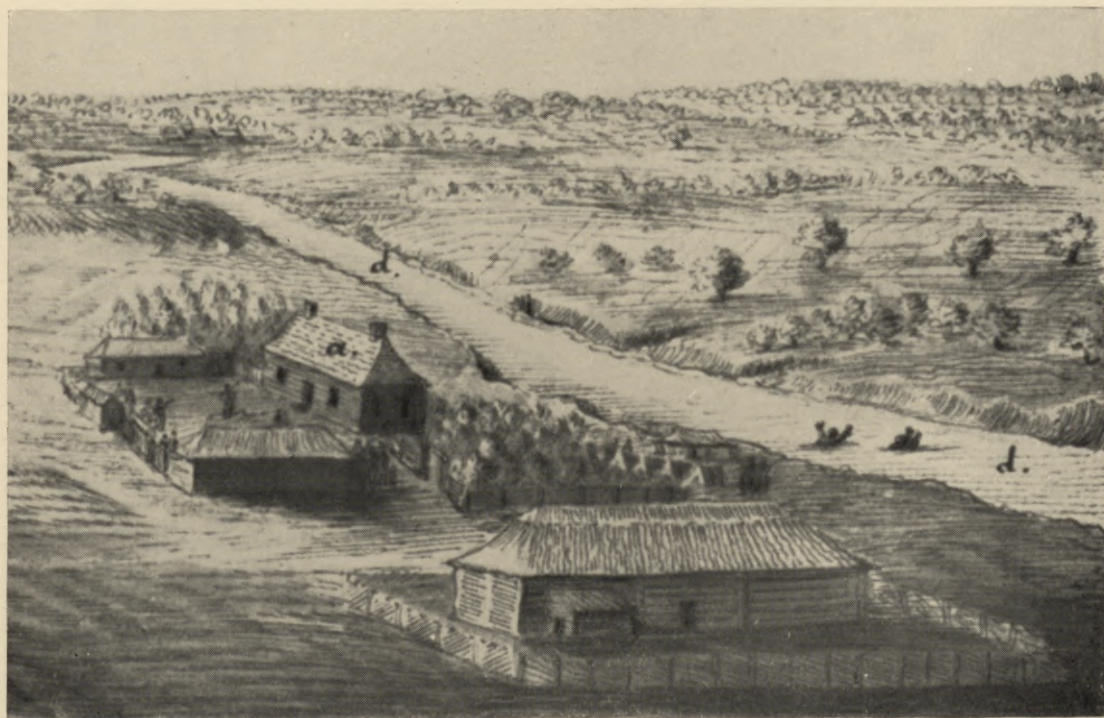
The Pamuša Manor in 1702. (A detail of battle picture on the Mūsa (d) river). The picture shows the timber buildings of the Pamuša Manor, grouped around the living house (a). The drying-kiln has been built at some distance from the house to insure fire protection. Split-rail fence around the buildings.
