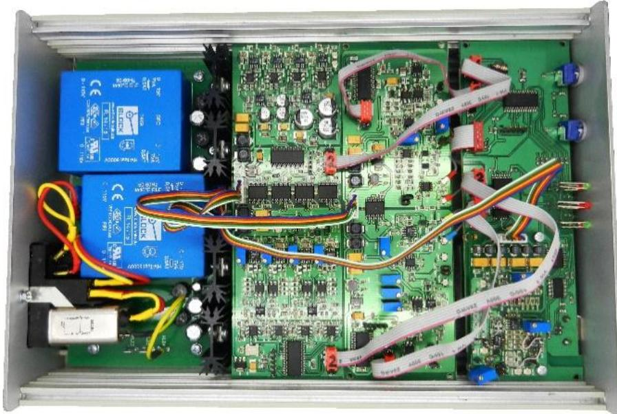
**Intelligent multi-frequency dielectrometer for non-destructive testing of quality of non-metallic materials**
