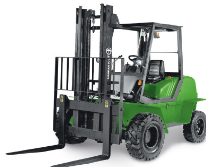
Fig. 1. Forklift with the “classic” design – engine, gearbox and front drive wheels.
