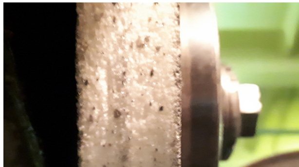
Fig. 6. The condition of the surface of the wheel after processing
