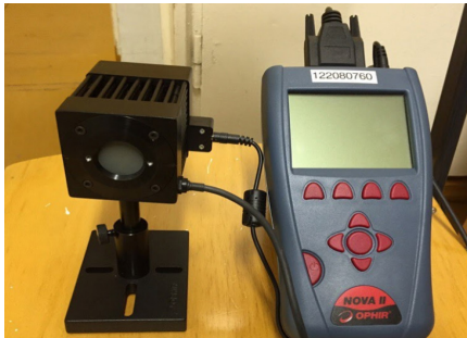
Fig. 8. Power measurement sensor OPHIR F150A-BB-26
