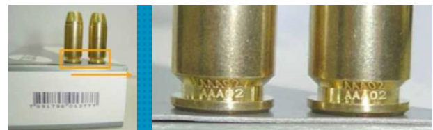
Fig. 1. Brass ammunition cartridge laser marking. [2]
