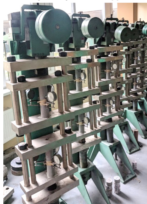
Fig. 5. Creep lever test stands with foamed concrete specimens inserted.
