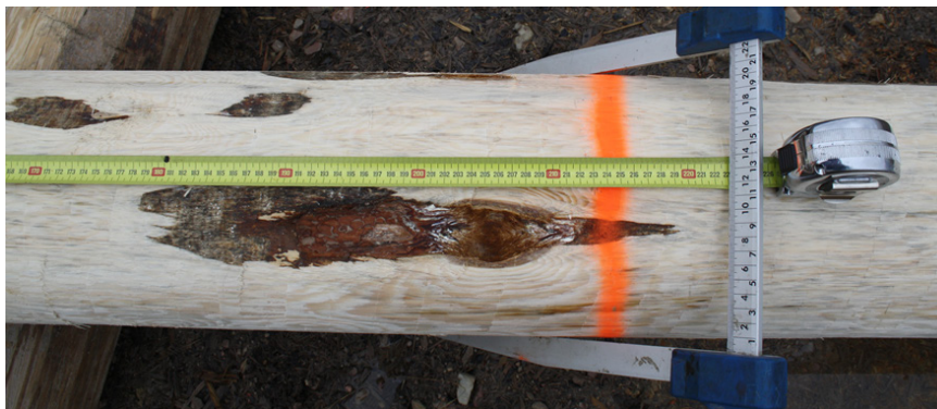
Fig. 3. The measurement of conk location place dimensions on infected wood pole surface
