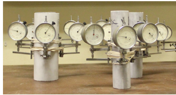
Fig. 3. Specimens prepared for shrinkage testing.
