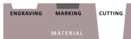
Fig. 1. Schematic view of laser cutting, engraving and marking processes.
