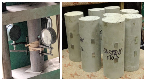
Fig. 2. Specimens prepared for creep testing.
