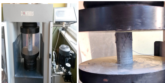
Fig. 1. Specimen compressive strength test.
