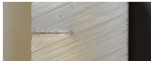
Fig. 5. qualitative marking of the material at a power of 20w and a speed of 25mm/s.
