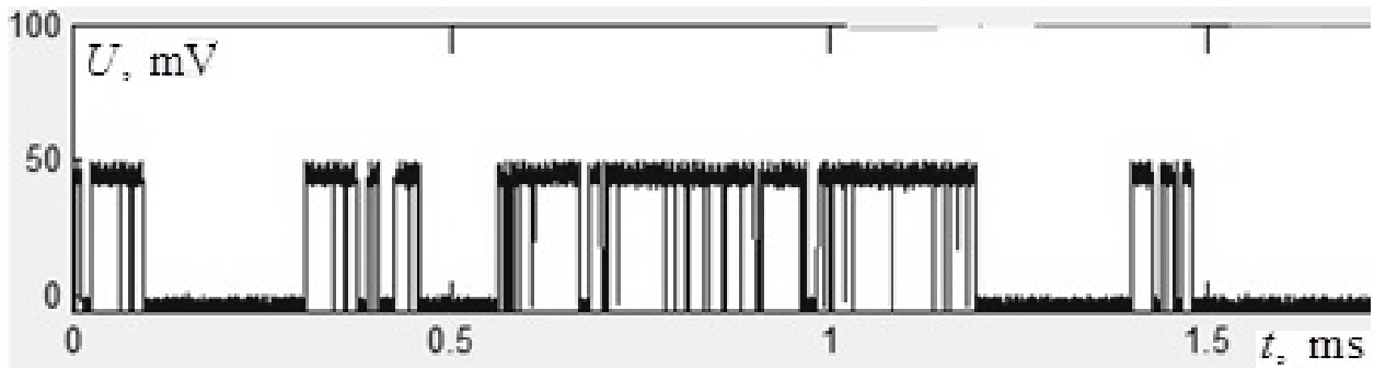
Fig. 2. Oscilloscope of pulse current through reverse biased p-n -junction at avalanche breakdown type B
