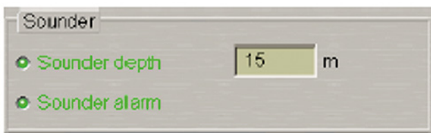
Fig. 4.12. Sounder alarm window (TRANSAS NTPro 5000).
