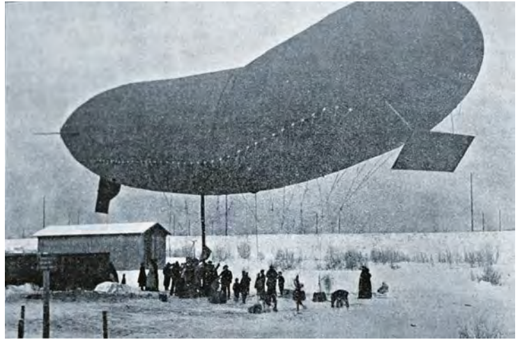
24 Forssman's soft-type dirigible, built by Riedinger in Augsburg, Gerstenhofen 1912.
