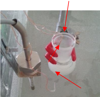
Fig. 2.1. Eutectic mixture in constant temperature water bath with thermocouples.
