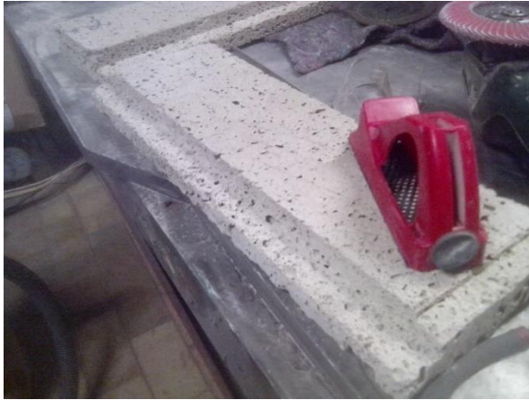
Fig. 3.31. The boards are easy to shape with hand tools.
