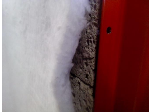
Fig. 3.32. The sheet prototype material is embedded in the outer insulation layer.
