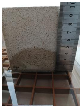
Figure 1. One of the prepared samples during the capillary water absorption test.
