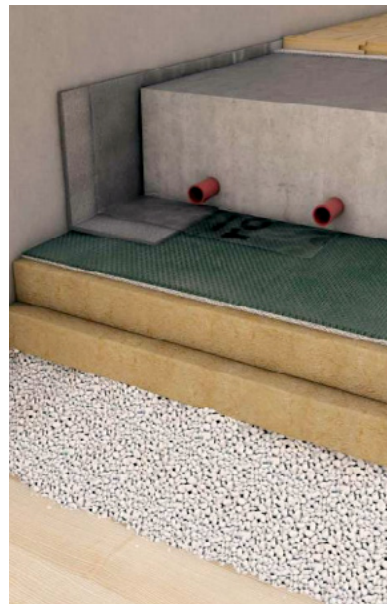
Fig. 3.48. Green waterproof membrane on top of the insulation (Rothoblaas, 2019).
