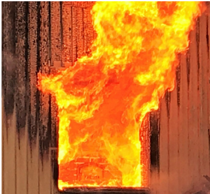
Fig. 3.21. The flames spread from the broken window to the wooden facade.
