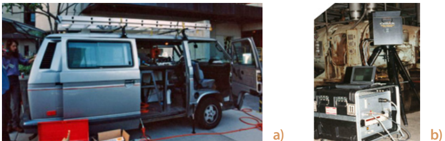
Fig. 6.2. Cyrax laser scanning system: a) prototype, b) model Alpha (Cheves, 2014).
