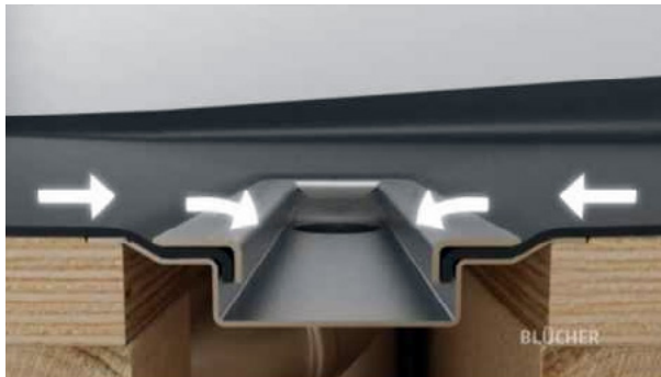
Fig. 3.51. Drains and membranes (Blucher, 2020).
