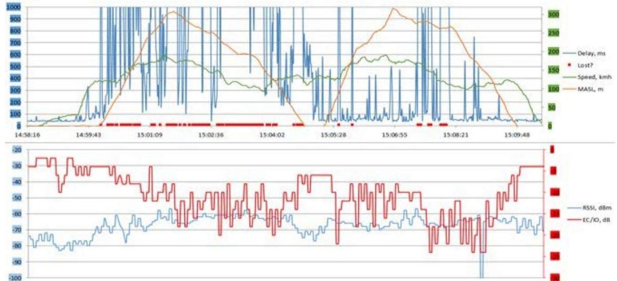
Fig. 3.1. Network performance during ground roll, two laps with one take-off and one go-around, as well as one landing.
