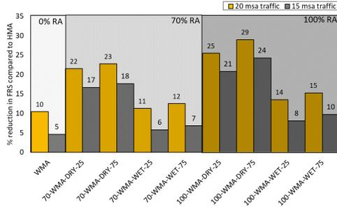
Fig. 8.7. Percentage reduction in fossil resource scarcity (in kg of oil eq) compared to the HMA mixture
