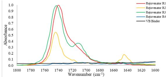
Fig. 3.2. Normalised FTIR spectra for all the rejuvenators used in this study
