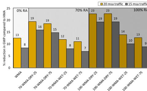
Fig. 8.4. Percentage reduction in GWP (kg CO<sub>2</sub> eq) compared to HMA mixture
