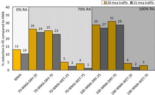
Fig. 8.5. Percentage reduction in freshwater ecotoxicity (kg 1,4-DB eq) compared to the HMA mixture
