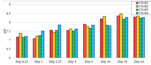
Fig. 6.4. pH value of leachant samples during the horizontal dynamic surface leaching test
