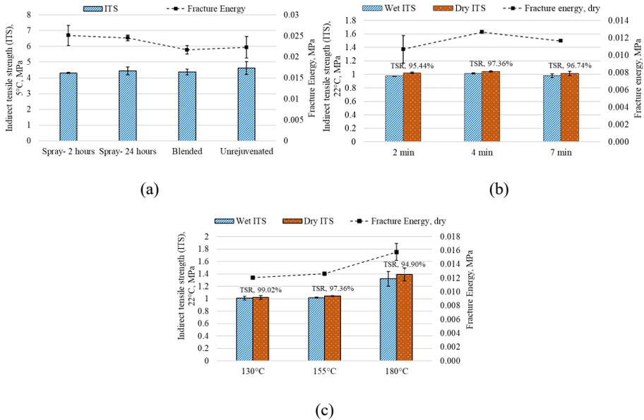
Fig. 4.2. ITS results for different (a) rejuvenation methods; (b) mixing time; (c) mixing temperature. The error bars indicate one standard deviation.
