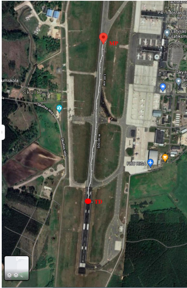
Fig. 5.4. Data on braking path received from GPS receiver.
