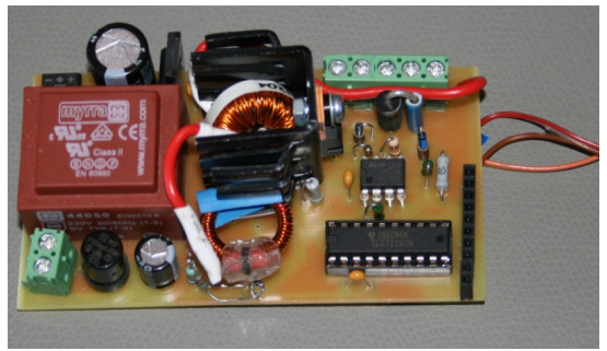
b) dimmer with integrated control module.
