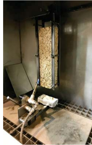
Fig. 4.7. MOC testing according to Standard LVS EN ISO 11925-2.
