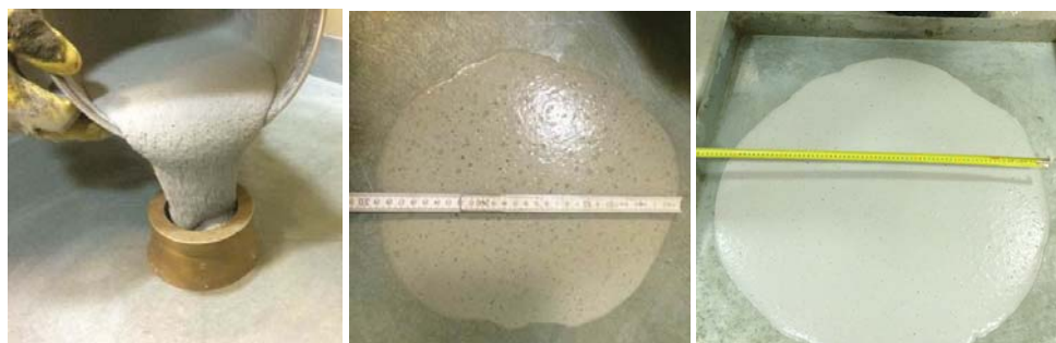
Fig. 2.11. Concrete consistency measurements for concrete M1.
