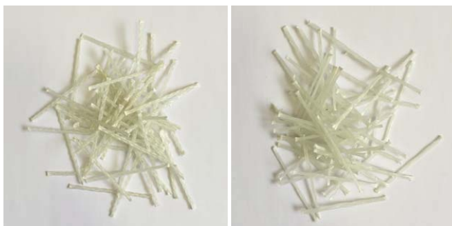
Fig. 2.7. Composite glass fibres: GF4 and GF5 (from the left).
