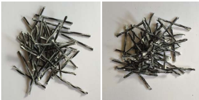
Fig. 2.9. Hybrid composite fibres: CG1(on the left) and GC1 (on the right).
