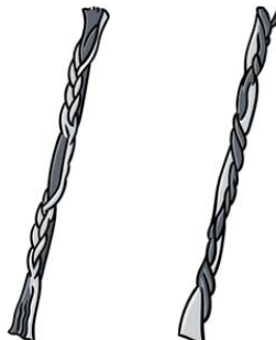
Fig. 2.10. Schematic representation of hybrid composite fibres: CG1 and GC1 (from the left).
