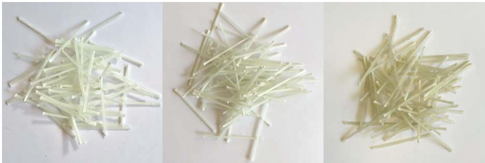
Fig. 2.6. Composite glass fibres GF1, GF2 and GF3 (from the left).
