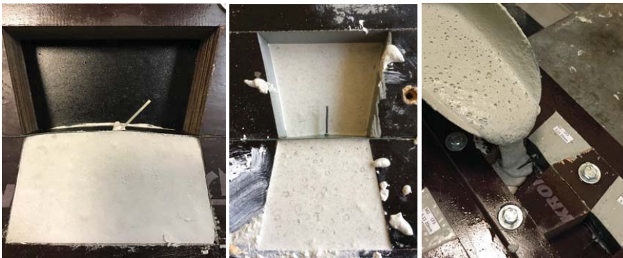
Fig. 2.13. Fibre configurations in depth (first and second on the left), moulds filling with concrete (on the right).
