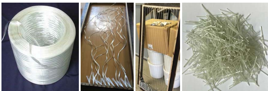
Fig. 2.1. Raw fibre transformation stages into the composite fibre.
