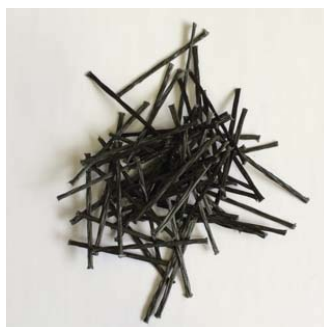
Fig. 2.4. Braided composite carbon fibre CF3.
