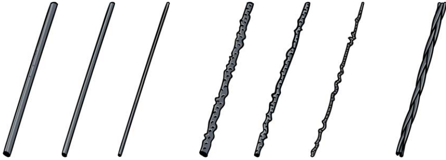
Fig. 2.5. Schematic representation of composite carbon fibres: CF1, CF1-A, CF1-B (smooth); CF2, CF2-A, CF2-B (rough), and CF3 (interlaced) from the left.
