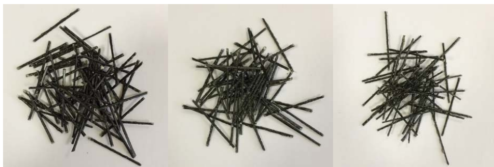
Fig. 2.3. Composite carbon fibres: CF2, CF2-A and CF2-B (from the left).
