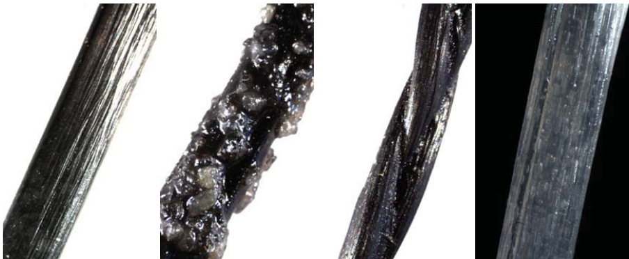
Fig. 2.20. Composite carbon and glass fibres with smooth surface, rough surface and braided shape: CF1, CF2, CF3, and GF2 (from the left).
