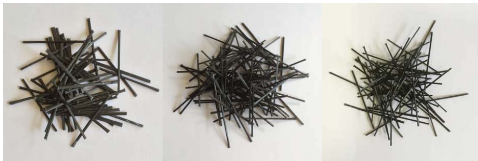
Fig. 2.2. Composite carbon fibres: CF1, CF1-A and CF1-B (from the left).
