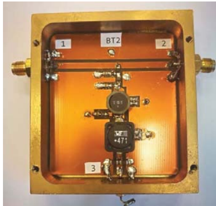
Fig. 3.7. Filter prototype with enclosure.
