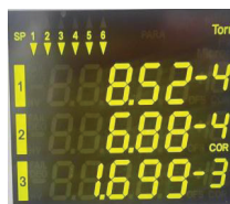
Fig. 2.3. Ionization vacuum gauge HPG 400 pressure measurements with argon correction.
