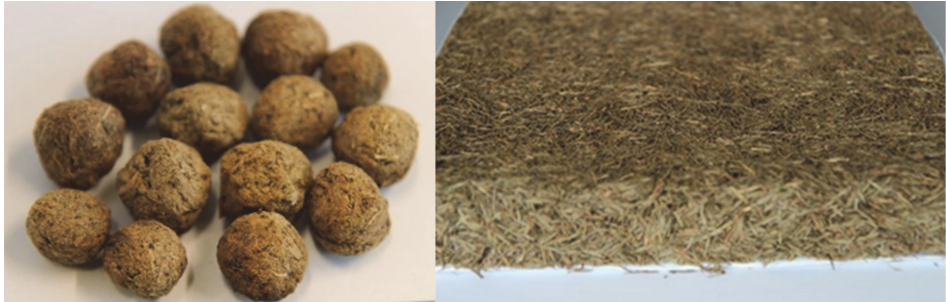
Fig. 4.2. Samples of thermal insulating materials – granular (picture on the left) and plate (picture on the right).
