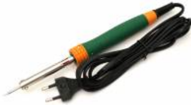
Figure 95: A soldering iron with the conical tip.
