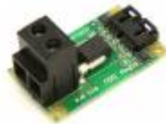
Figure 36: Analog current meter module 0–50 A.
