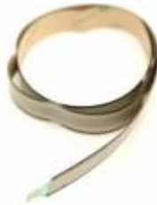
Figure 21: Force sensitive resistor (FSR).
