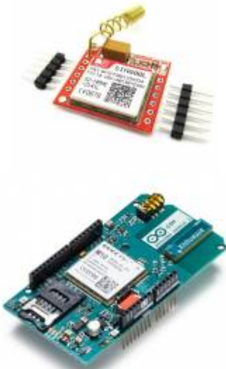
Figure 266: Sample GSM hardware for IoT prototyping.
