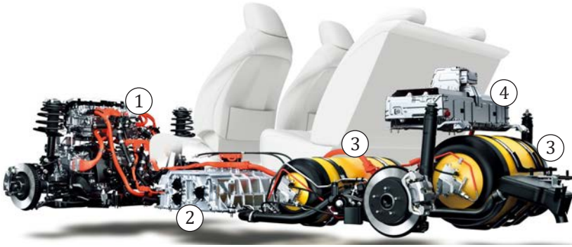
Fig. 4.3. Composition of Toyota Mirai hydrogen car chassis: 1 – electric motor; 2 – block of fuel cells; 3 – hydrogen high pressure tanks; 4 – electric battery.
