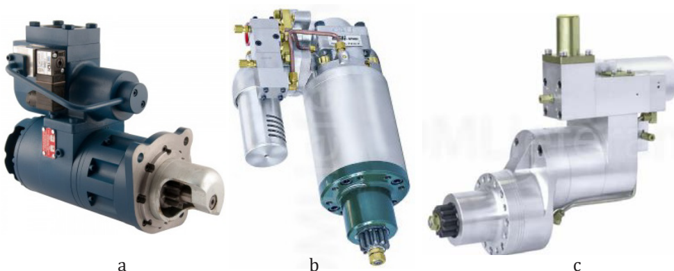
Fig. 4.33. Exterior of pneumatic starters: a, b – rotary type; c – turbine type.
