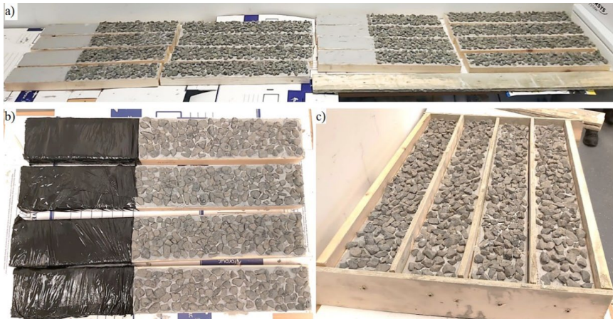
Fig. 5.1. Specimen producing stages: a) 16 specimens after the glue has dried; b) wrapping 40 % of the specimen end in a PE film to ensure the defect; c) specimens placed in the molds.
