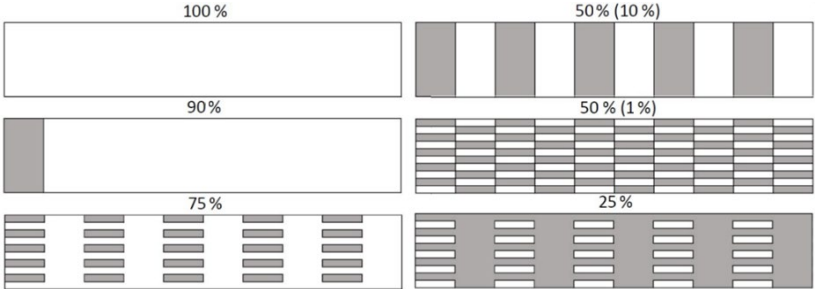
Fig. 2.3. Timber-to-concrete connection scheme with good-quality glued areas (white) and non-glued areas (grey), where many areas form non-glued defects with a length equal to 10 % of the total specimen length.
