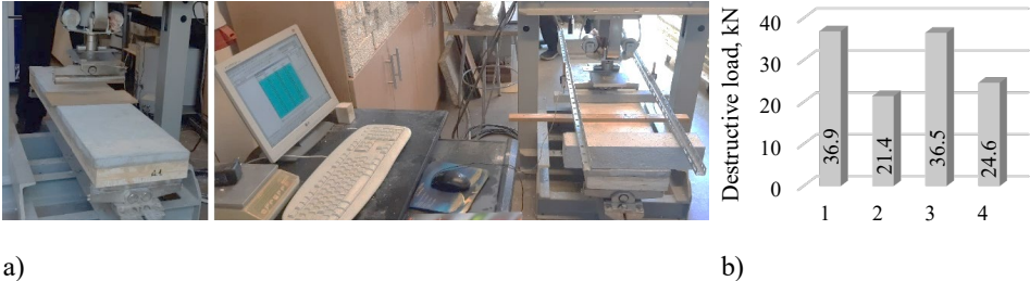
Fig. 5.8. a) The process of loading TCC specimens in three-point bending; b) values of destructive loads for CLT-concrete specimens with and without fibres (1 and 2 – specimens without fibres; 3 and 4 – specimens with fibres).
