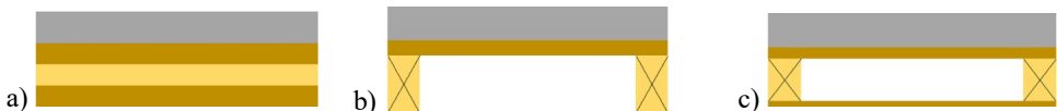
Fig. 4.1. Timber-concrete composite slab structural solutions: a) with CTL panel; b) with timber beams; c) with a ribbed plywood panel.
