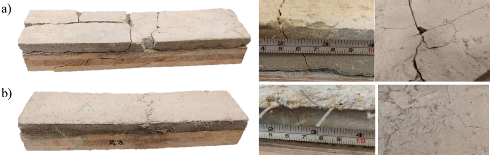
Fig. 5.9. Full failure scene, nature and development of cracks for TCC specimens: a) without fibres; b) with fibres.
