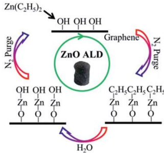
Figure 1.1. Deposition mechanism of ZnO nanostructures using atomic layer deposition method [26]
