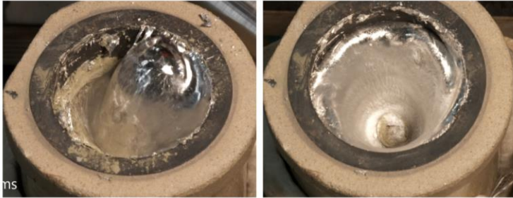
Figure 12 Stirring of a semi-solid ( \sim 610 °C) A360 alloy - intense surface deformations caused by a PM stirrer on the side of the crucible (left), vortex flow caused by a PM stirrer below the crucible (right).
