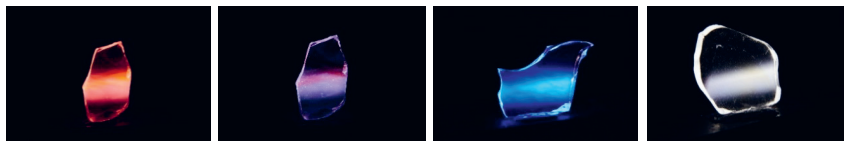
Figure 3.4. Photographs of luminescence in oxyfluoride glasses: a) \text{Eu}^{3+} ions ( \lambda_{\text{ex}} = 320 \text{ nm} ); b) \text{Eu}^{3+} and \text{Eu}^{2+} ions ( \lambda_{\text{ex}} = 350 \text{ nm} ); \text{Eu}^{2+} ions ( \lambda_{\text{ex}} = 350 \text{ nm} ); \text{Tb}^{3+} and \text{Eu}^{3+} ions ( \lambda_{\text{ex}} = 350 \text{ nm} )
