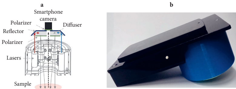
Figure 3.1 Optical beam in the illumination device of three laser lines (a), the external appearance of the device in a set with a smartphone (b) [P1, K6, K7, K8, K9]
