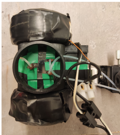
(b) Coils with the holder for experiments with vertical magnetic field that is parallel to the microfluidics chip.
