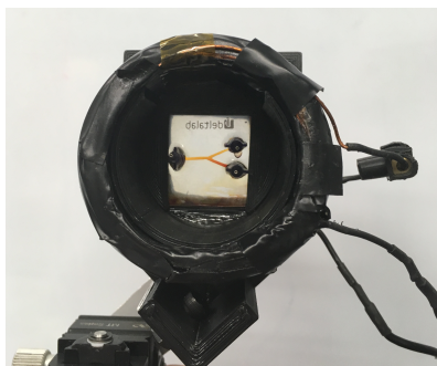
(a) Coils with the holder for experiments with horizontal magnetic field that is perpendicular to the microfluidics chip.
