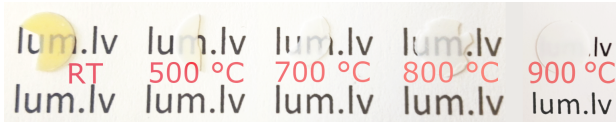
Figure 4.4: Pressed pellet (1 mm thickness) with no annealing (RT) and annealing at 500°C, 700°C, 800°C and 900°C temperatures (right).
