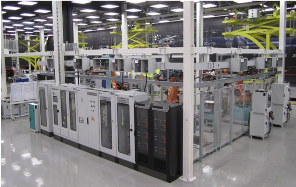
Fig. 4.1. DC microgrid realization as an automotive manufacturing cell for experimental analysis (Publication 5).
