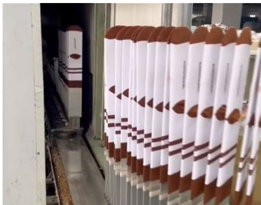
Fig. 4.11. Finishing hydrothermal treatment of socks [36].
