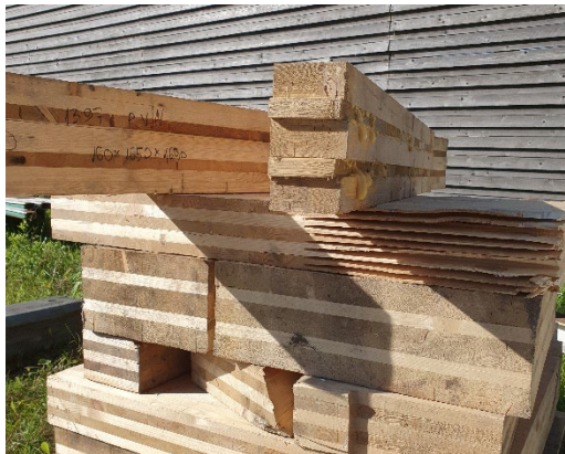
Fig. 1. Cross laminated timber non-reusable cuttings.
