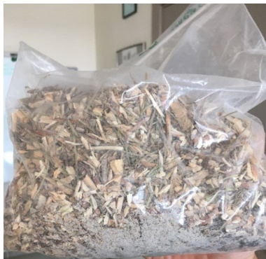
Fig.2.2. Biomass as received from logging site.
