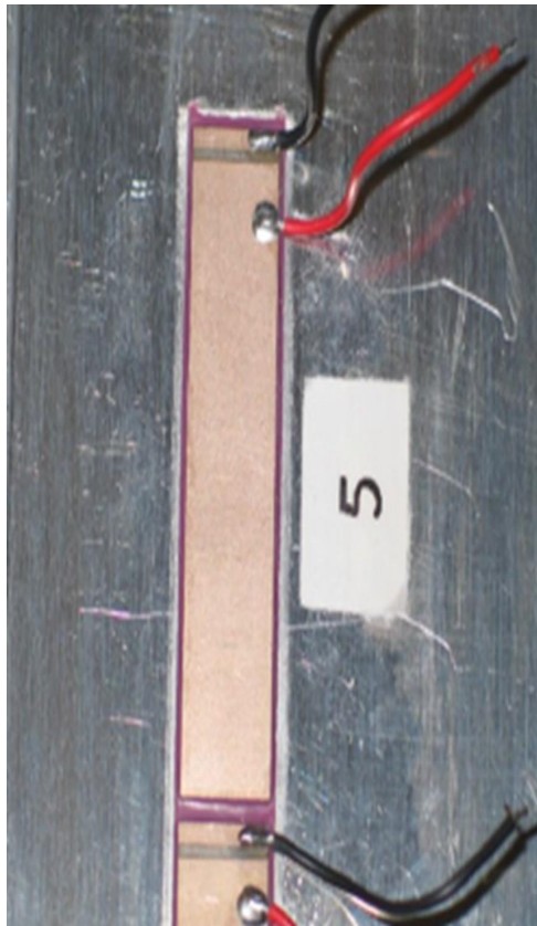
Fig. 2.4. View of the Piezoelectric transducer (PZT) number 5 before (left) and after (right) fatigue test and cracks evaluation by penetration method.
