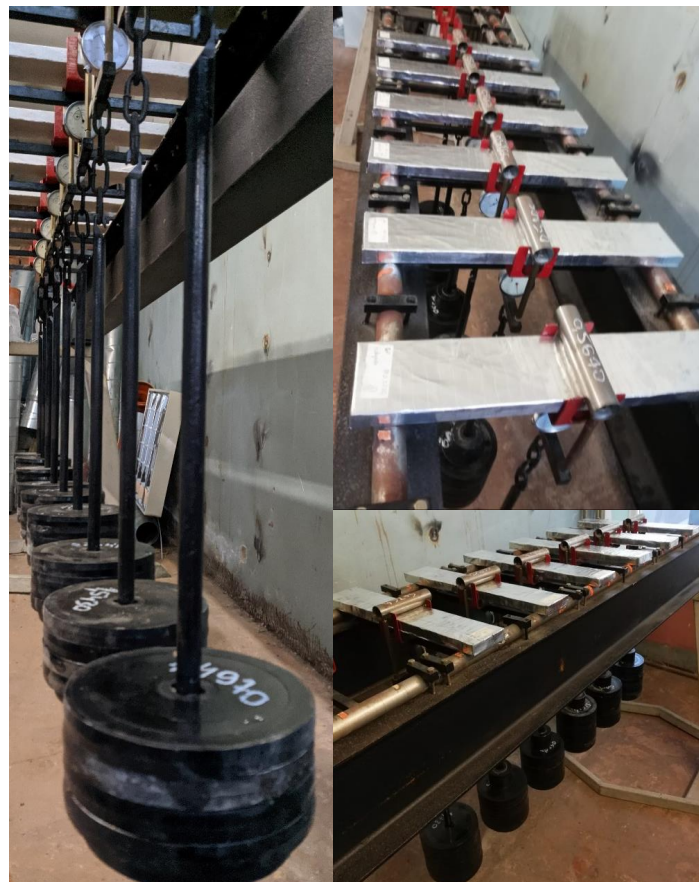
Figure 7. Setup and testing of long-term deflection strain in three-point bending.
