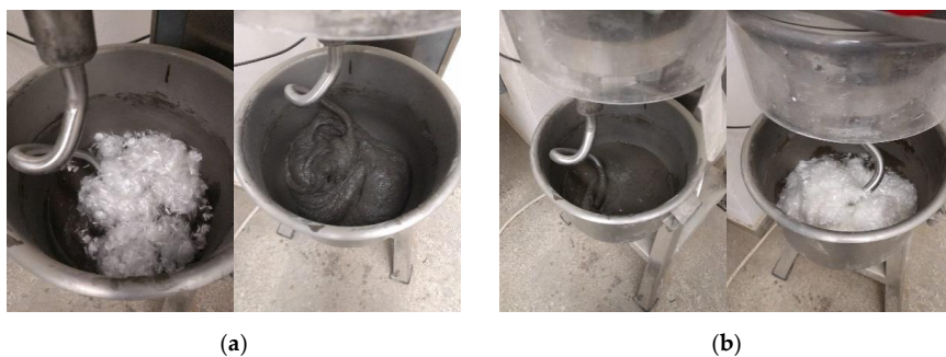
Figure 1. Geopolymer composite mixes, which were reinforced with 1% (a) and 5% (b) polypropylene fibers.
