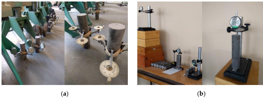
Figure 3. Prepared creep test specimens (a) and shrinkage specimens (b).
