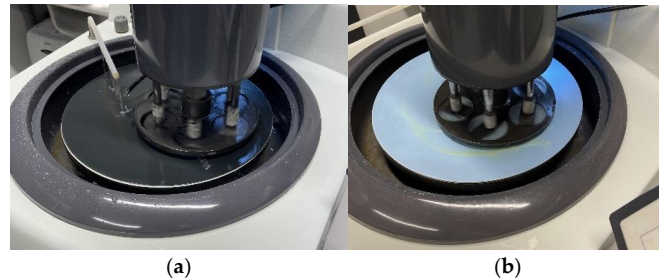
Figure 9. Geopolymer composite polished section specimen polishing with sandpaper (a) and polishing paste (b).
