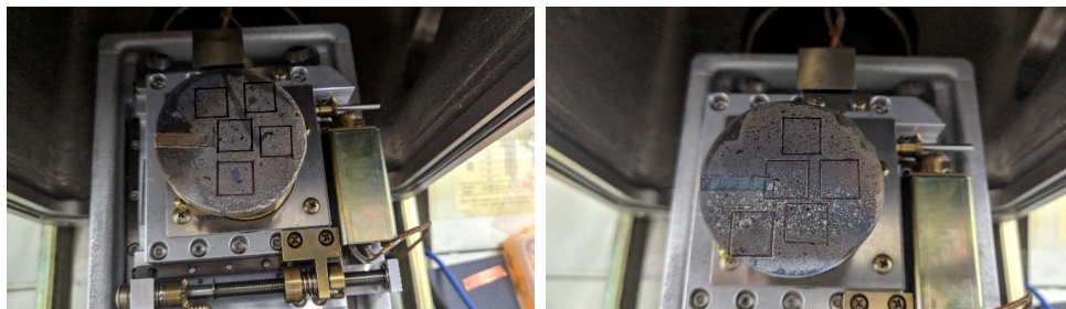
Figure 4: Specimen cross-section division into zones
