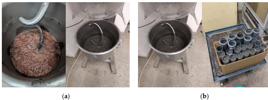
Figure 2. Geopolymer composite mixes, which were reinforced with 1% steel fibers reinforced (a) and plain (b).
