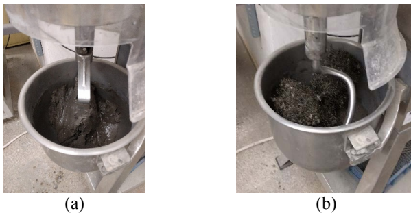
Figure 1: Plain geopolymer (a) and recycled tire steel cord reinforced geopolymer (b) concrete
