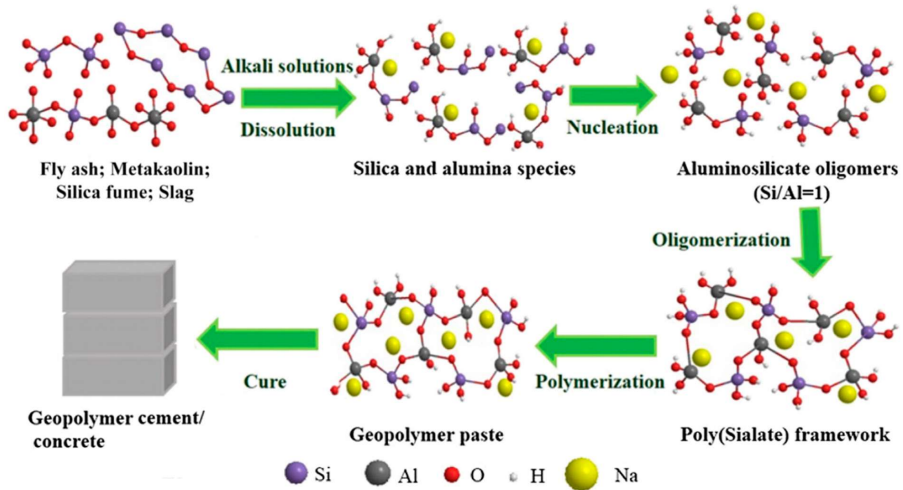
Fig. 9. Fly ash-based geopolymer cement/concrete chemical development scheme[148].
