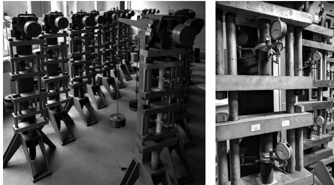
Fig. 2. Test setup for creep and elastic modulus tests.
