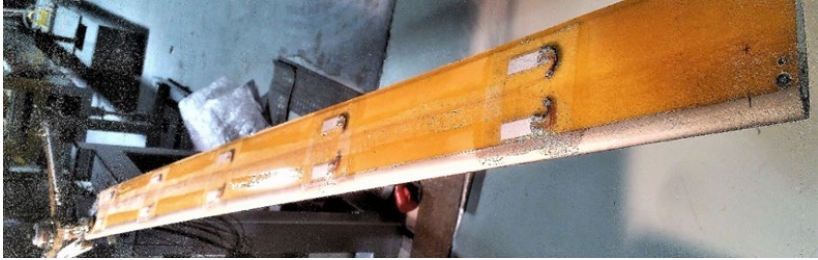
Fig. 4.11. Integrated array of deformation sensors and wiring.
