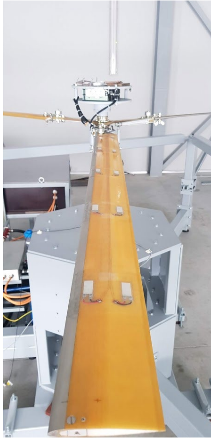
Fig. 4.5. Blade with piezo film sensors and measurement system.
