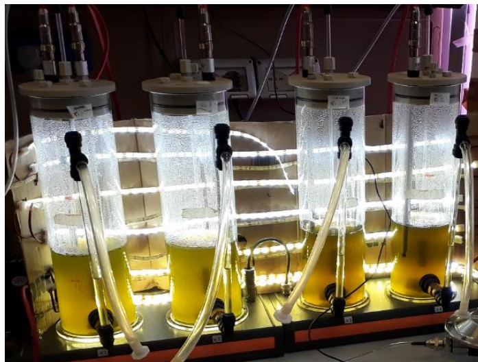
Figure 2.1. Experimental setup with photobioreactors at the beginning of growth tests.
