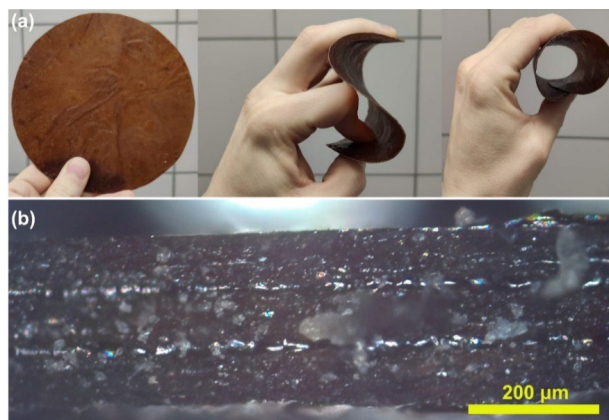
Figure 3.30. (a) Three-layer laminate prepared with 4:2:1:1 as an adhesive for hemp paper sheets. (b) Optical microscopy image showing 3 layers of laminate composite.
