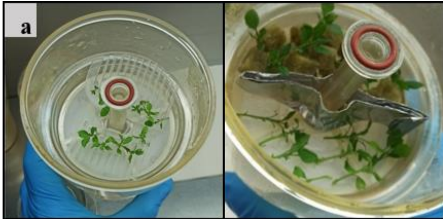
Figure 1. Supports used to maintain the explants in vertical position. a) plastics slots, b) RITA ® divided into two sections (cubes and no support).
