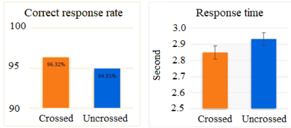
Figure 10. The average correct response rate (left) and response time (right) for crossed and uncrossed disparity present on a flat-panel display.
