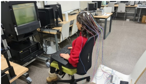
Figure 5. The experiment set up and electrodes placement.
