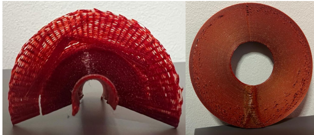
Fig. 5.11. Example of cylindrical printing without flow control and with manual percentage.
