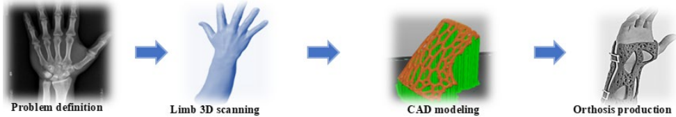
Fig. 1.1. 3D-printed orthosis production stages.
