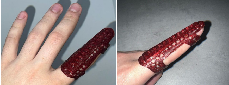
Fig. 6.10. 5-axis printed example of finger orthosis with a 45° layer infill.
