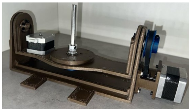
Fig. 6.8. Additional A and B axis printing table mechanism from PA12 nylon material.
