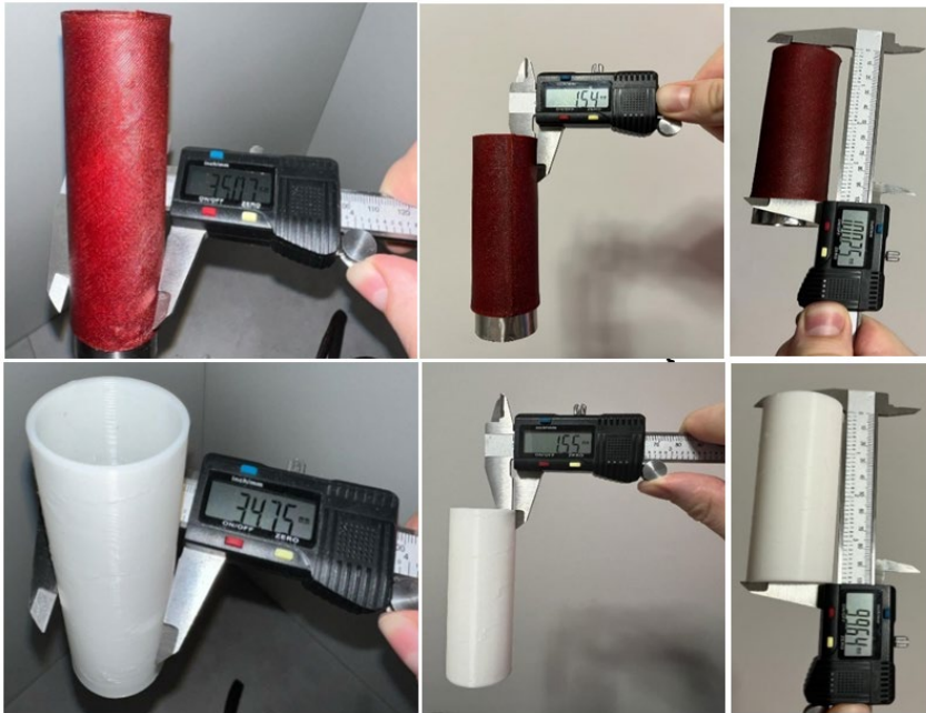
Fig. 5.28. Comparison results of printed sample sizes of PLA material.
