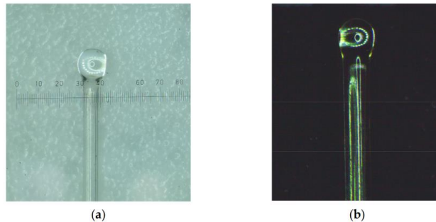
Figure 1. The obtained microsphere samples: (a) microsphere with a diameter of 380 \mu\text{m} ; (b) microsphere with a diameter of 200 \mu\text{m} .
