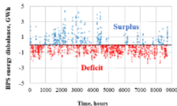
Fig. 6. BPS 2050 energy imbalance after energy import/export procedures (reserve stations are not used, 2 mil. EVs are used)
