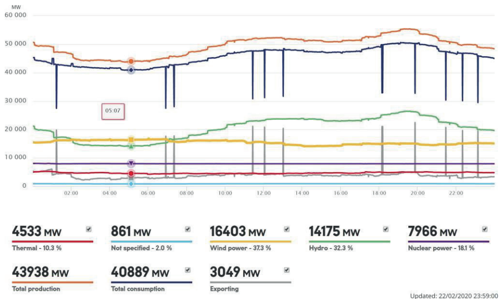
Fig. 1. Balance by production sources of the Nordic and Baltic power system on February 22, 2020.
