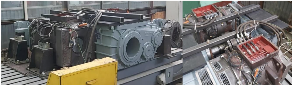
Fig. 5.33. MGU placement on the test platform under mutual load.
