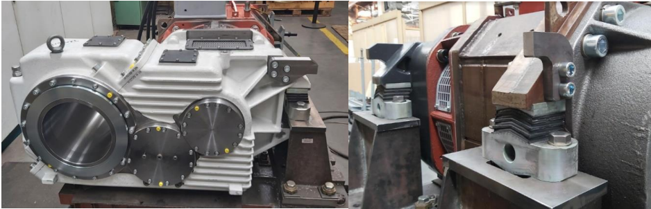
Fig. 5.32. MGU placement on the test platform to determine its own vibration.
