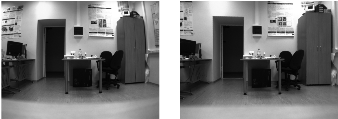
Figure 4.15. Correction of radial lens distortions in Bumblebee camera using spatial transformation IP.
