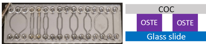
Figure 3. Finished OSTE 322 device on the left and the side view of the device on the right.
