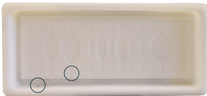
Figure 2.2.1. Printed mould without air escape holes, circles indicated defects.
