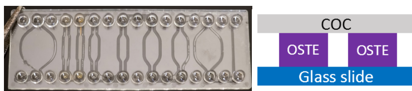
Figure 3.1.6. Finished OSTE 322 device on the left and the side view of the device on the right.
