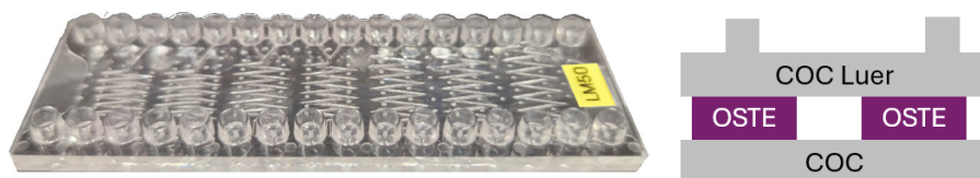
Figure 3.2.4. Finished device on the left and the side view of the device on the right.
